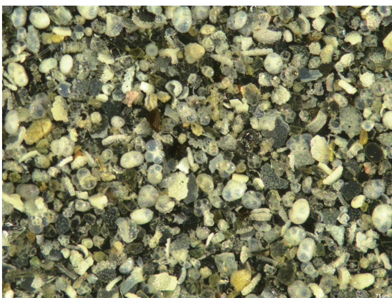
Image A2 True-color stereo microscope image of marine microfossils with particle sizes of minor axis lengths between 0.038 mm and 0.063 mm.
