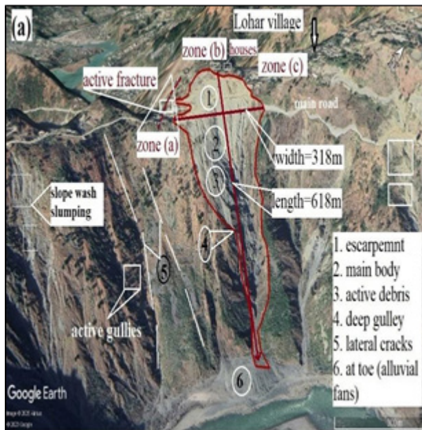
Figure 2: The above Google Earth picture (a) shows the aerial view of western section features of Lohar Gali slope; (b) shows the circular failure steeply dipping strata, escarpment slope adjacent to main highway with striations of sliding over blocks, infrastructure at high risk with risk zonation (a,b,c).
