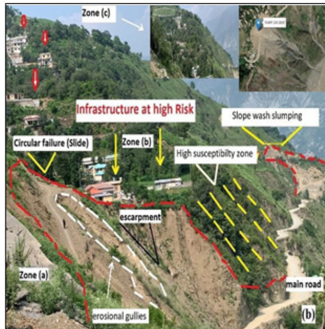
Figure 2: The above Google Earth picture (a) shows the aerial view of western section features of Lohar Gali slope; (b) shows the circular failure steeply dipping strata, escarpment slope adjacent to main highway with striations of sliding over blocks, infrastructure at high risk with risk zonation (a,b,c).
