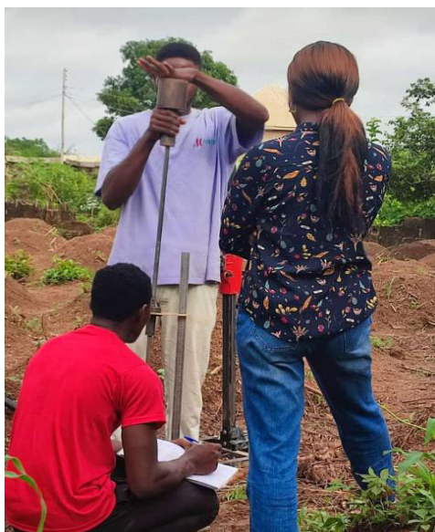
Figure 2 Dynamic Cone Penetrometer test on a proposed site for a bungalow at Ebonyi state, Nigeria by Mapref Geotechnical Ltd.
