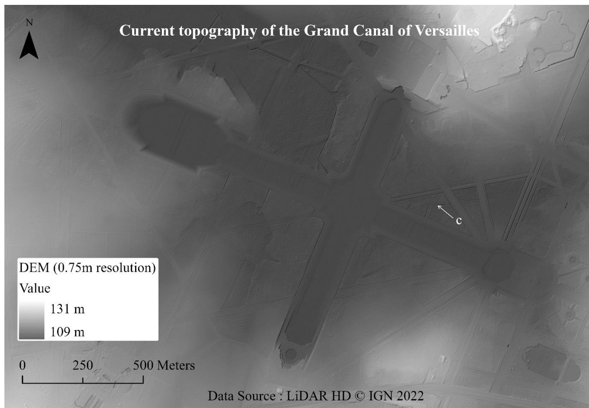
Figure 2. Digital Elevation Model of the Grand Canal in Versailles, computed from LiDAR aerial data acquired by the French Geographical Institute (IGN) in 2022. The heights reference is the average sea level at Marseille.
