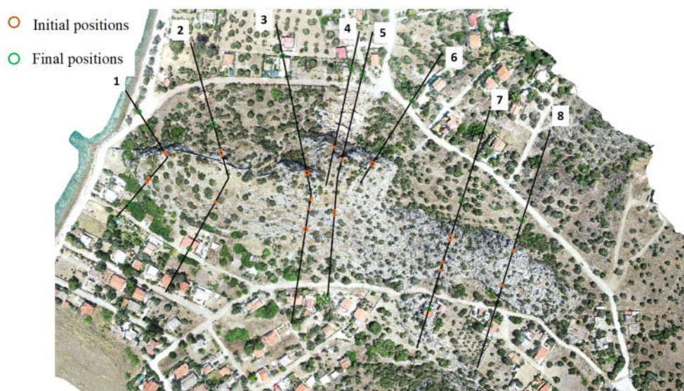
Figure 4 Trajectories (initial and final positions) of the rock blocks simulated in the 2D analyses.
