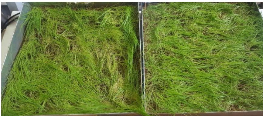
Figure 10. Erosive changes of slopes with vegetation, polymer-improved slope (left side), and natural slope (right side)
