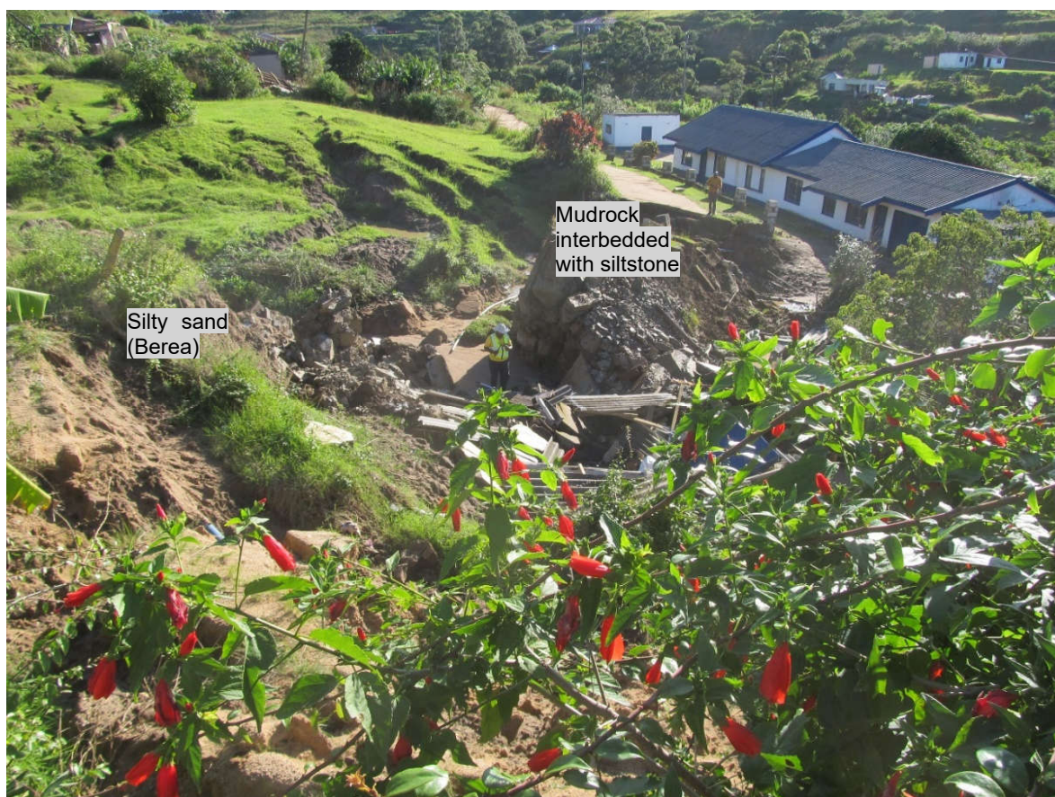
Figure 3. Local geology is characterised by Vryheid Formation mudrocks and siltstone overlain by Berea-type sands.
