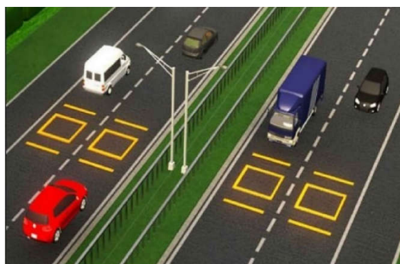
Figure 5. Illustration of the Induction Loops on a road (Federal Highway Administration, U.S. Department of Transportation, 2006)
