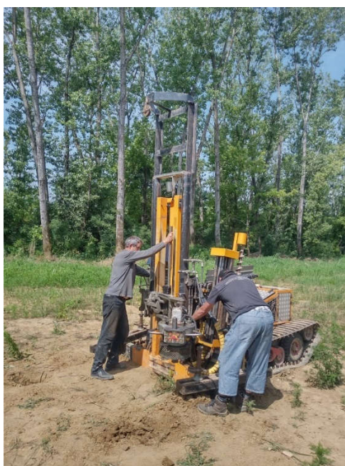
Figure 1. Cone Penetration Testing in the area of Petrinja
