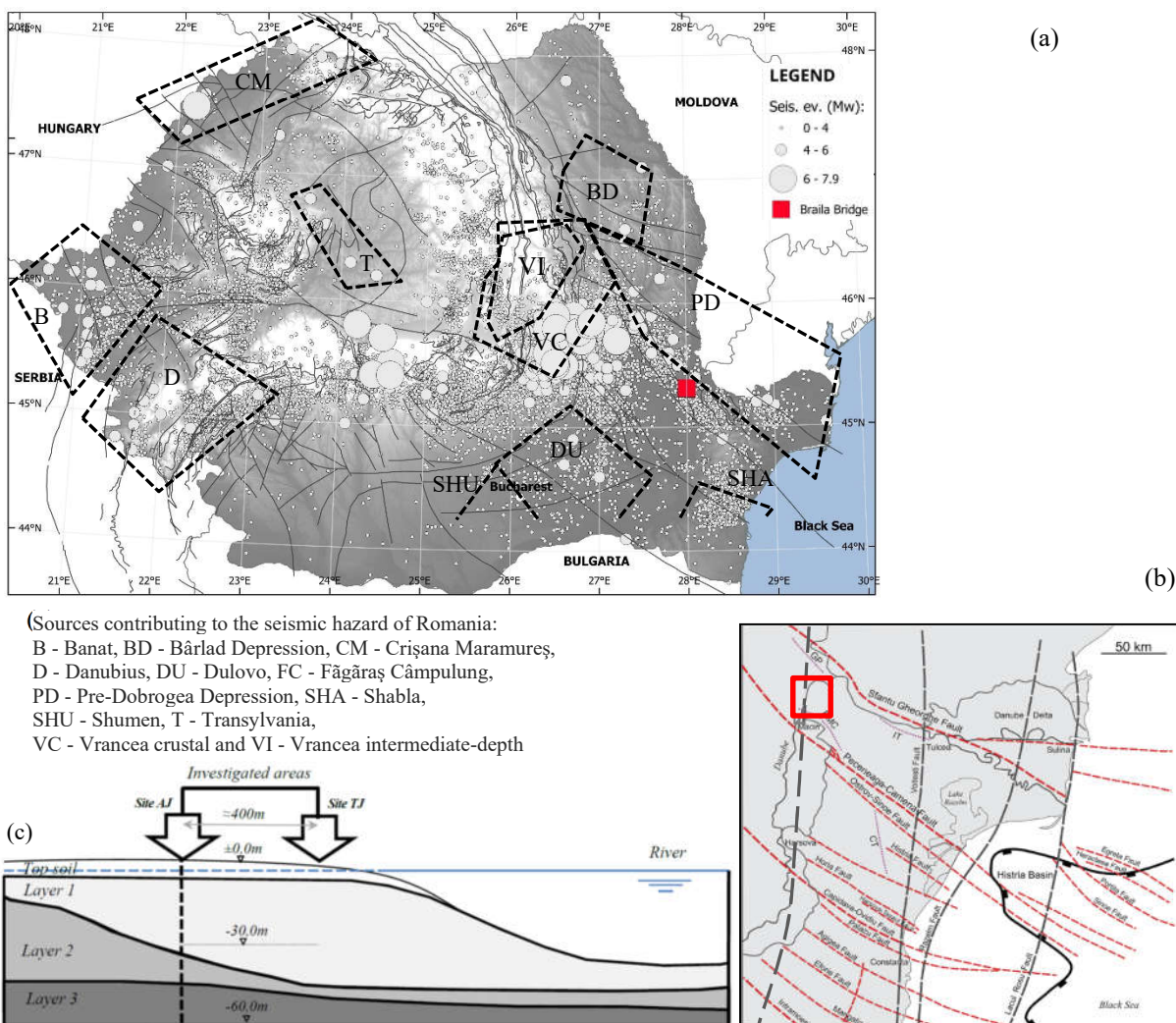
Figure 1. (a) Location of the sites on the seismic map of Romania (compilation after Popa et.al, 2022 and Văcăreanu et.al., 2016); (b) Tectonic map of Western sector of Black Sea (Oaie et al. , 2016); (c) Sketch of Holocene sedimentary structure of approximate 60m depth.
