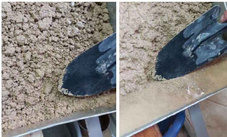
Figure 9. Eroded soil in 180 minutes of rainfall for polymer-improved slope (left side) and natural slope (right side).
