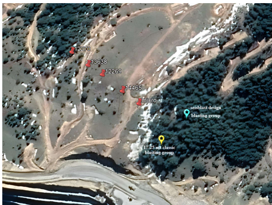
Figure 1. Group blasting locations and seismograph locations (Seismographs: micro,14465,12269,13638,12270)
