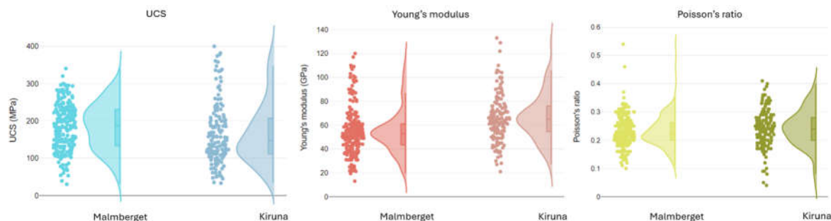
Figure 3 Summarised distribution of all tested samples for UCS, Young's modulus and Poisson's ratio.
