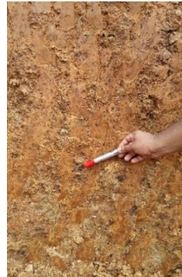
Figure 3 Iron-manganese concretions in deeply weathered Madhupur Clay
