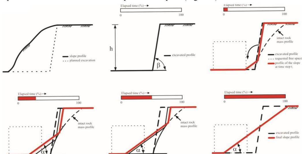
**Figure 1.** Formation of a steep slope from the initial time to its final transformation. Jelušič et al (2024)
