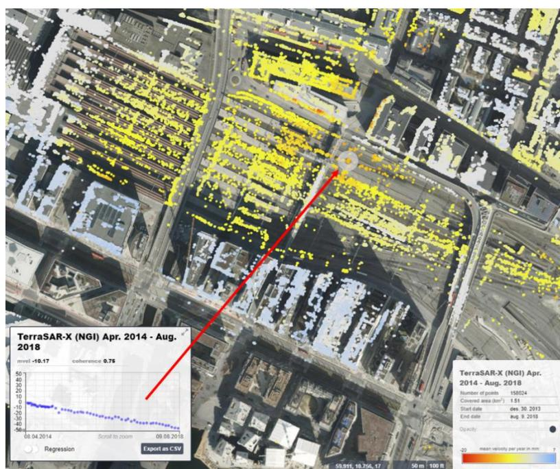
**Figure 1: Example of InSAR measurements over the track area of Oslo Central Station. Color-coded measurement points show the mean ground velocity between Apr. 2014 and August 2018. The time-series shows the displacement history for the same period. The data was processed from a TerraSAR-X image stack in staring spotlight mode (resolution <1m) using a Permanent Scatterer algorithm. (see <https://insarkart.ngi.no/malte/oslopublic>)**
