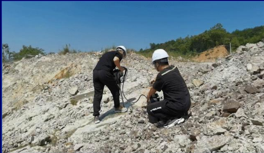
Coring & making samples at the site
