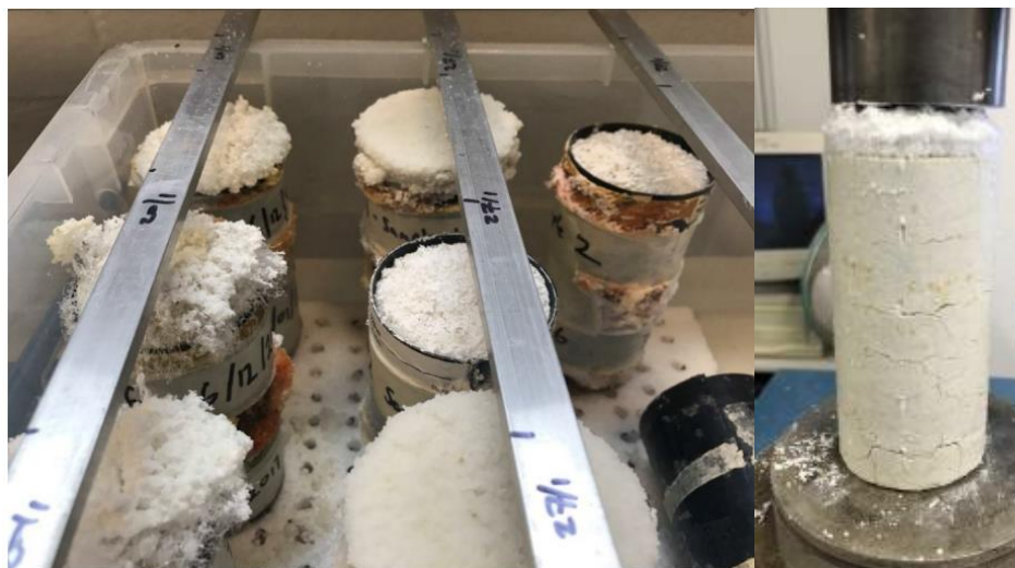
Figure 4. Salt formation in MgO mixes and specimen damage (here, MgO-GGBS mix) before UCS testing
