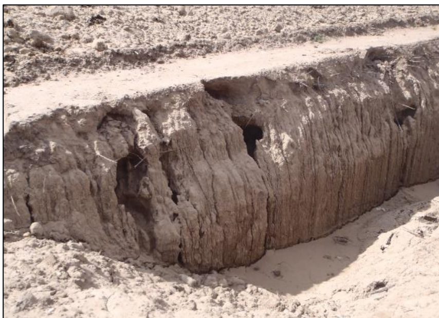
Figure 10. Piping Erosion of Sodic Soils Within Open Pipeline Excavations
