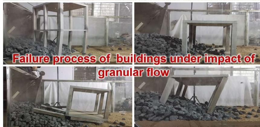
Model tests of building damage under landslide impact
