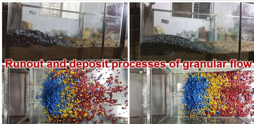
Model tests of landslide runout behaviors
