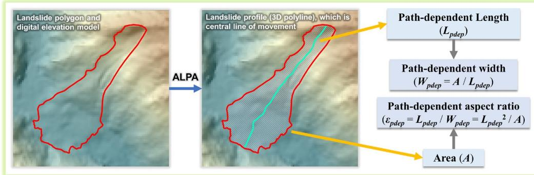
**Fig. 3** Conceptual overview of the new approach for measuring path-dependent landslide length, width and aspect ratio (i.e.,  $L_{pdep}$ ,  $W_{pdep}$  and  $\varepsilon_{pdep}$ ) based on landslide profile (i.e., central line of movement).
