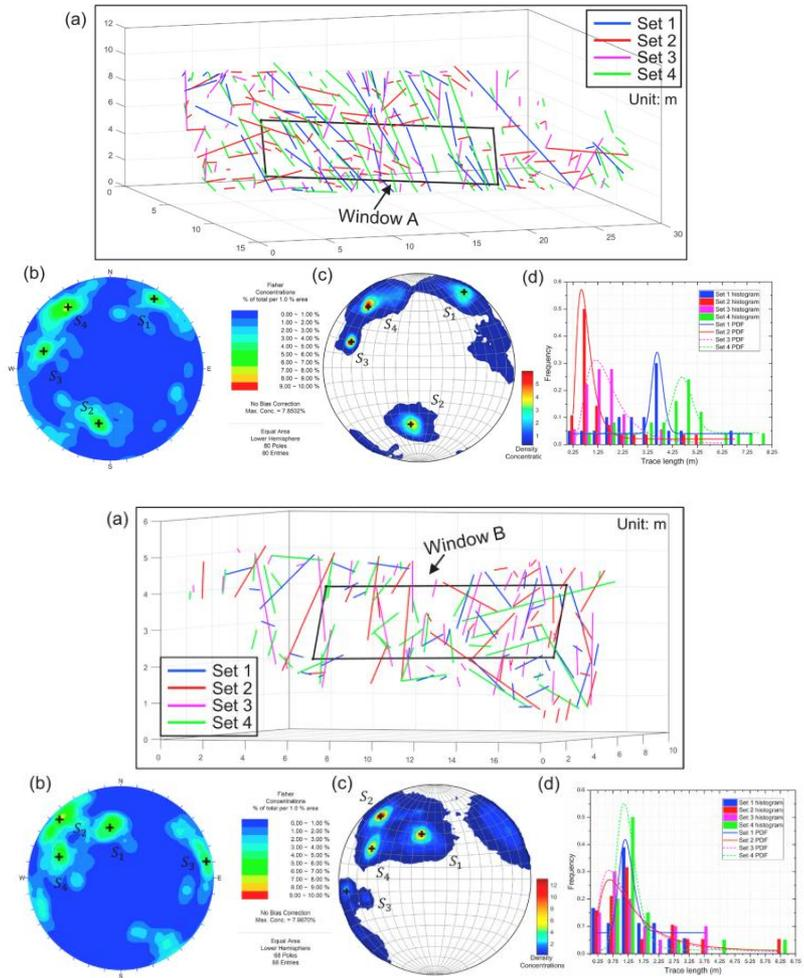
To achieve the window sampling from digital trace mapping, a rectangle window was placed on the slope face plane. The locations of four vertices stay consistent with the actual window in the field survey.
