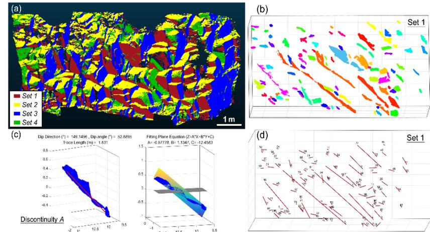
PCM-DDN method that presents the existing rock block reconstruction of full-scale rock exposure, in accordance with the mutual intersection relationship of discontinuities. This procedure describes the initial state of rock blocks in detail and reveals the structural complexity of the entire rock surface.
