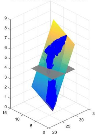
one joint orientation and trace length calculation
