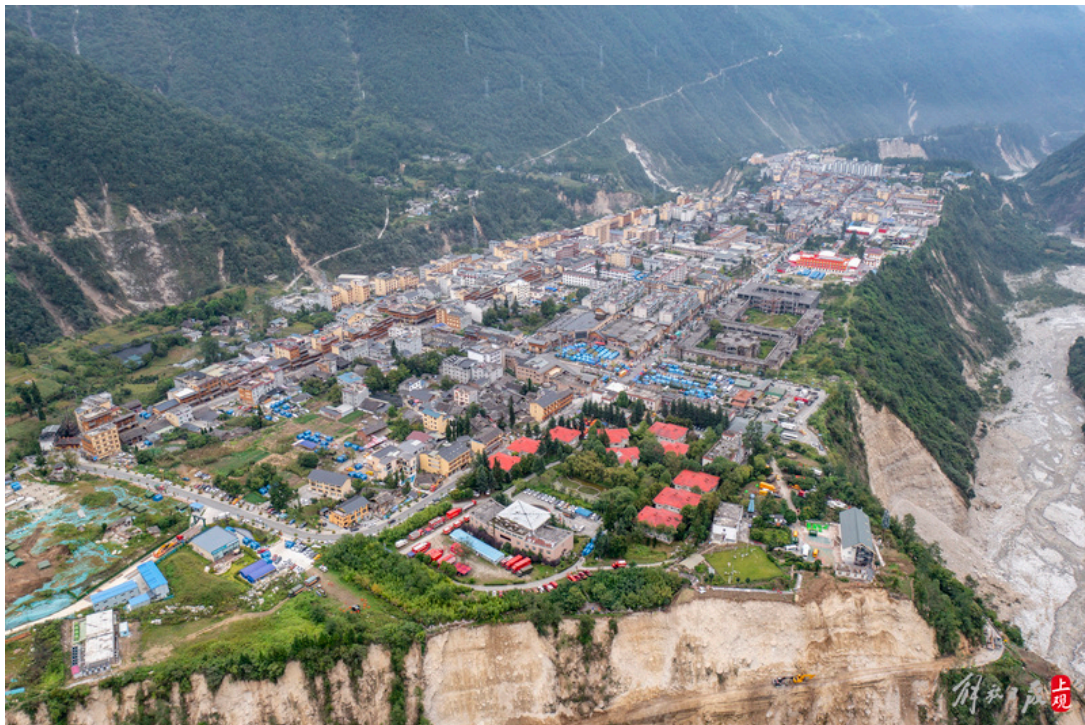
Fig.4 The collapse characteristics of Moxi Mesa edge after '9.5' Luding Ms 6.8 earthquake
