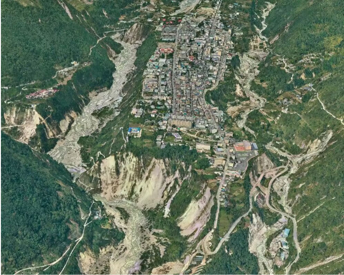
Fig.5 Distribution characteristics of geological disasters around Moxi platform after '9.5' Luding Ms 6.8 earthquake
