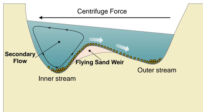
**Fig. 6 The Flying Sand Weir (Feishayan) can drain out sand into the outer stream by hydraulic principles.**
