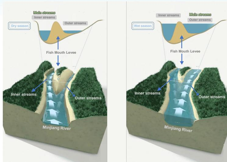
**Fig. 5 The Fish Mouse Levee (Yuzui) ensures that the inner stream carries approximately 60% of the river's flow into the inner stream (to Chengdu Plain) during dry season. While during flood, this amount decreases to 40% to protect the people from flooding.**
