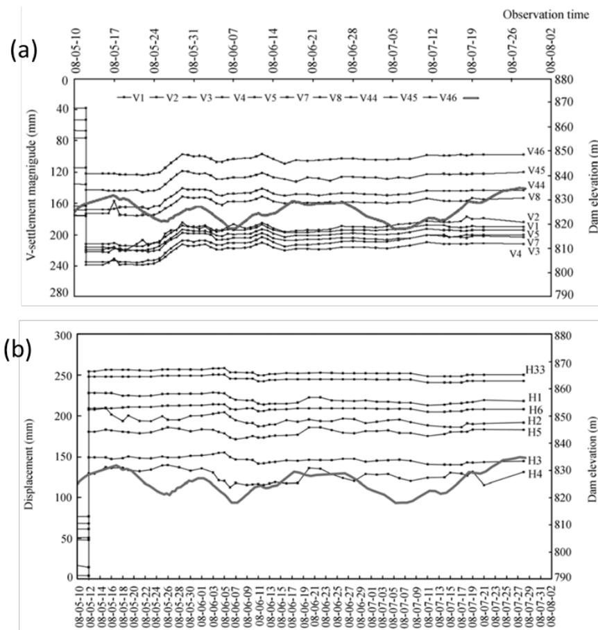
**Fig. 13** The interior observation results of the dam. (a) Settlement graph of the observation points at El. 760m; (b) Horizontal displacement graph of the observation points at El. 760.0 m (positive in downstream direction).
