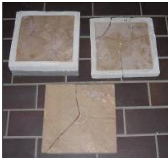
Figure 21: Test results illustrating the influence of the setting : the tile alone (bottom) doesn't resist a drop of 35 cm, while the same tile embedded in a mortar of 2cm thickness breaks at 60cm (upper right). If the mortar is settled on a concrete slab, no damages are observed after a drop of 200cm (upper left)
