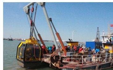
Demonstration of offshore cone penetration test
